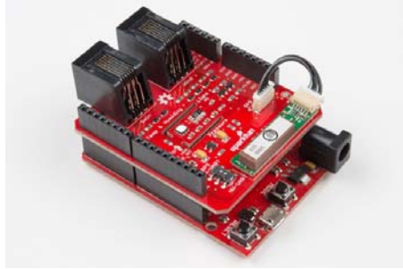
The Arduino Weather Shield attached to a Photon RedBoard.
