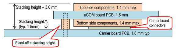
Figure 16 – uCOM Board Mounting on Carrier Board, Stacking Height
