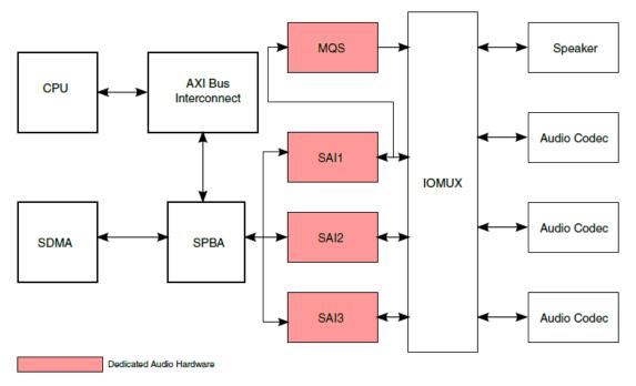
Figure 5 – Audio Subsystem Block Diagram
