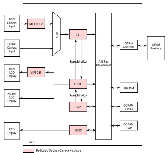
Figure 4 – Structure of Display and Graphics Subsystem
