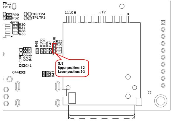
Figure 19 – Location of SJ8 on COM Carrier Board
