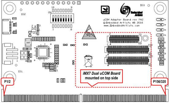
Figure 8 - uCOM Adapter Board Pin Numbering, Top Side
