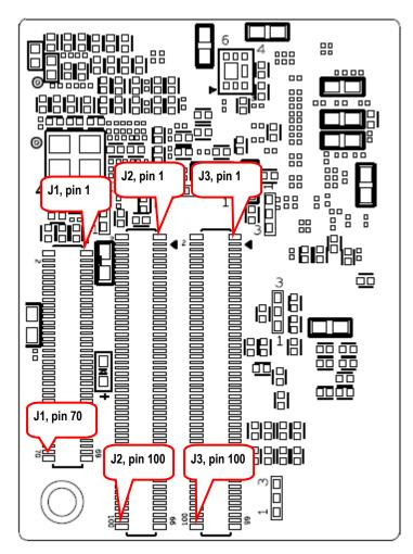
Figure 2 - EACOM Board Pin Numbering, Bottom Side
