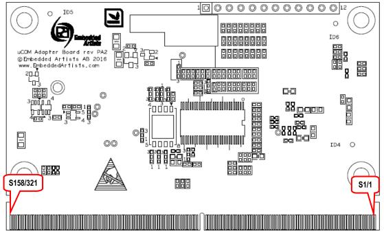
Figure 9 - uCOM Adapter Board Pin Numbering, Bottom Side
