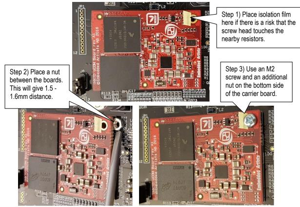
Figure 17 – iMX7 Dual uCOM Board Assembly
