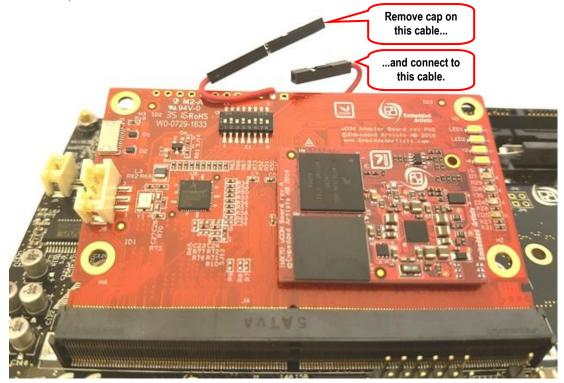
Figure 18 – uCOM Adapter Board with Special Cable
