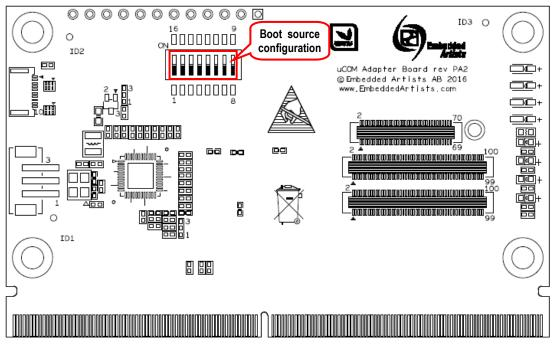
Figure 12 –uCOM Adapter Board Boot Control Slider Switches Location
