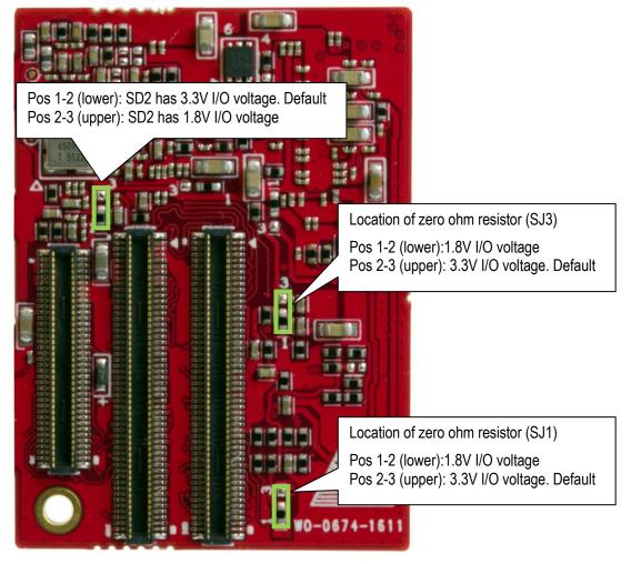
Figure 11 - iMX 7Dual uCOM Board, Bottom Side Photo
