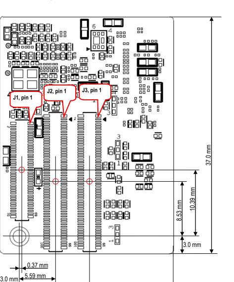
The picture below show the mechanical details of the *iMX7 Dual uCOM Board*. The outer measurement is only 27 x 37 mm. Note that the picture below is seen from the bottom side.
