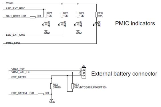
Figure 7 - Battery Integration to iMX7 Dual uCOM Board
