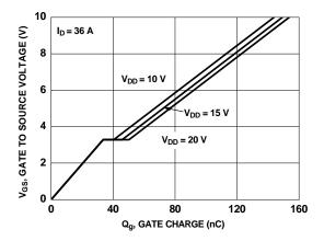
Figure 7. Gate Charge Characteristics
