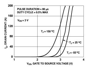
Figure 5. Transfer Characteristics
