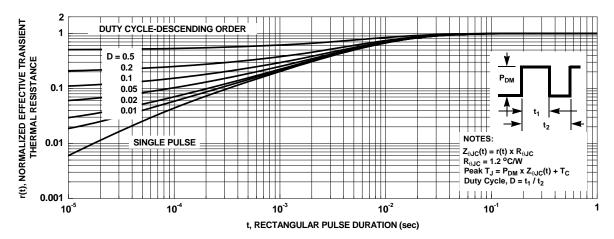
Figure 13. Junction-to-Case Transient Thermal Response Curve
