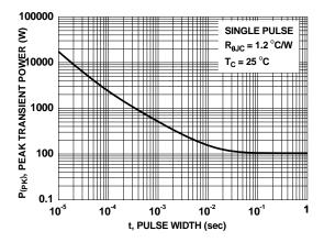
Figure 12. Single Pulse Maximum Power Dissipation
