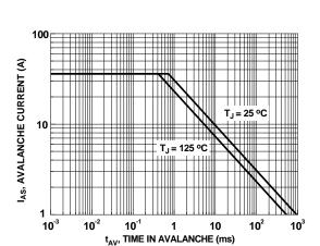
Figure 9. Unclamped Inductive Switching Capability
