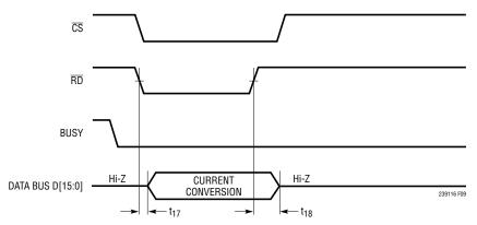
Figure 9. Read the Parallel Data After the Conversion
