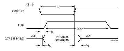
Figure 10. Read the Parallel Data During the Conversion
