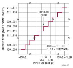
Figure 2. LTC2391-16 Two's Complement Transfer Function
