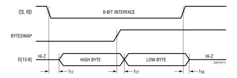
Figure 11. 8-Bit Parallel Interface Using the BYTESWAP Pin
