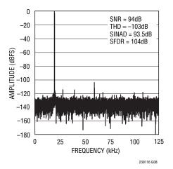
Figure 5. 16k Point FFT of the LTC2391-16,  $f_S = 250ksps$ ,  $f_{IN} = 20kHz$
