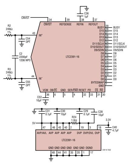
Partial Schematic of Demoboard
