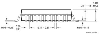
NOTE: 1. PACKAGE DIMENSIONS CONFORM TO JEDEC #MS-026 PACKAGE OUTLINE 2. DIMENSIONS ARE IN MILLIMETERS
