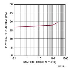
Figure 7. Power Dissipation of the LTC2391-16 Decreases with Decreasing Sampling Frequency
