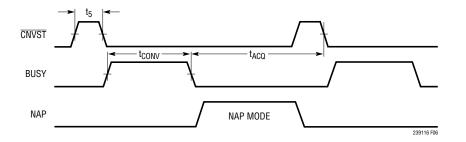
Figure 6. Nap Mode Timing for the LTC2391-16
