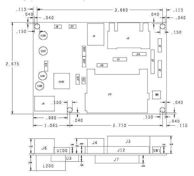
Figure A-1 Host Interface Board Dimensions
