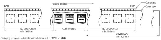
Projection 8.5 SSt 2014-09-16 BD 8.4 2013-12-11 SSt SSt SSt 8.3 2013-04-29 SSt Würth Elektronik eiSos GmbH & Co. KG EMC & Inductive Solutions SSt SSt 8.2 2012-12-05 Max-Eyth-Str. 1 2012-10-25 SSt BD 74638 Waldenburg Germany Pull-of force 2012-09-03 SSt BD Tel. +49 (0) 79 42 945 - 0 Tape width | 16 mm | 0,1 N - 1,3 N www.we-online.com 7.0 ME 2008-01-01 Tape width | 24 mm | 0,1 N - 1,3 N eiSos@we-online.com
