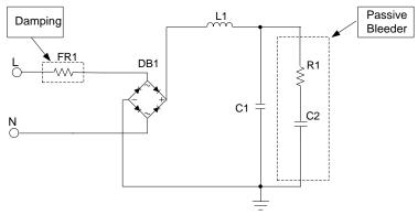
Figure 4. LED Driver Schematic with Passive Bleeder
