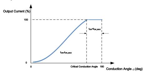
Figure 3. Dimming Curve
