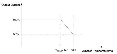
Figure 2. Thermal Foldback Waveform
