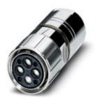
Cable connector, straight, Screw locking, M58, number of positions: 4+3+PE, type of contact: Socket, Crimp connection, shielded: yes, cable diameter range: 17 mm ... 25 mm
