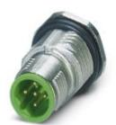
Sensor/actuator flush-type plug, with green contact carrier, 5-pos., M12 SPEEDCON, shielded, B-coded, rear/ screw mounting with M16 thread, with straight solder connection
