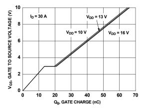
Figure 7. Gate Charge Characteristics
