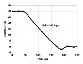
Figure 14. FDMS7560S SyncFET body diode reverse recovery characteristic
