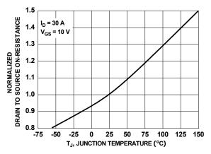
Figure 3. Normalized On-Resistance vs Junction Temperature
