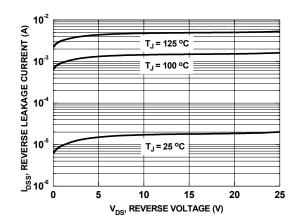
Figure 15. SyncFET body diode reverses leakage versus drain-source voltage
