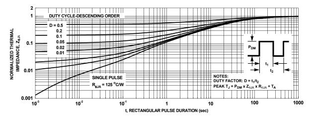
Figure 13. Junction-to-Ambient Transient Thermal Response Curve
