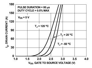
Figure 5. Transfer Characteristics
