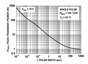
Figure 12. Single Pulse Maximum Power Dissipation
