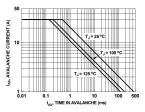
Figure 9. Unclamped Inductive Switching Capability
