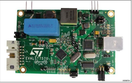
Figure 1. ST7570 demonstration board with outline dimensions
