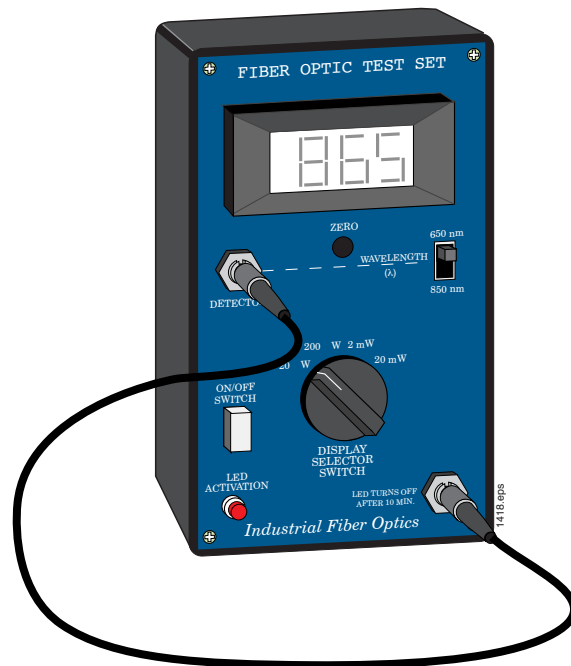
Figure 21. 1-meter fiber cable installed onto the Fiber Optic Test Set to take baseline measurements for characterizing an optical fiber coupler.
