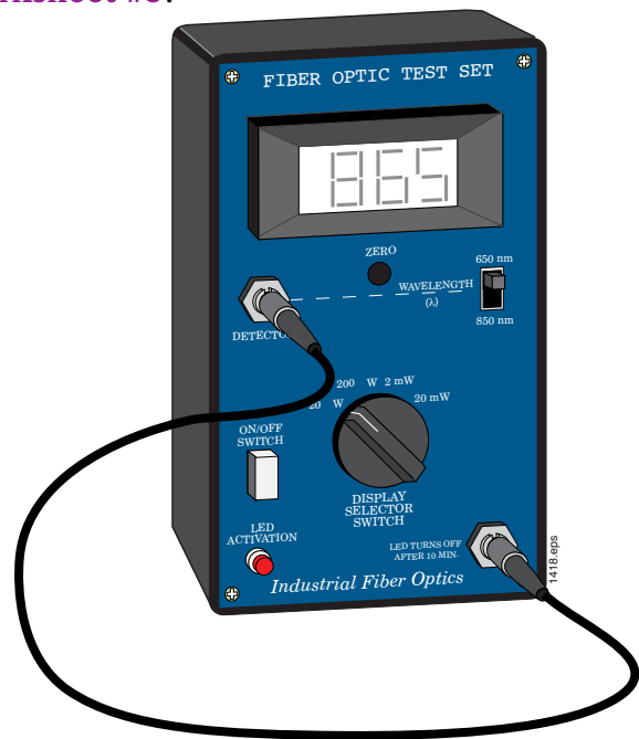
Figure 20. 3-meter fiber cable installed onto the Fiber Optic Test Set to take baseline measurements for characterizing the 2-meter fiber cable.
