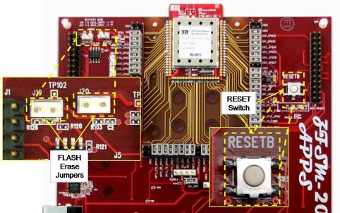
Figure 30 – Photo, EVB Details (FLASH Erase Jumpers & RESET)
