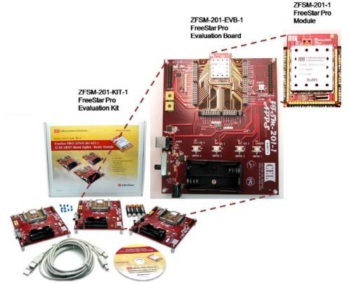
The main component in the Evaluation Kit is the **ZFSM201-EVB-1** FreeStar Pro Evaluation Board. The board serves as an interface, evaluation and development tool enabling the user to demonstrate, and evaluate the capabilities of the CEL **ZFSM-201-1**, FreeStar Pro Module. At the heart of the CEL **ZFSM-201-1** is the Freescale **MC13224V** Platform-in-Package (PiP) transceiver, a 32-bit ARM-based ZigBee radio module and a third-generation 2.4GHz IEEE® 802.15.4 platform.
