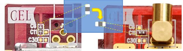
Figure 41 – Diagram, External Antenna Capacitor Change The PCB Trace antenna will no longer be connected and the MMCX Jack connector will be active.
