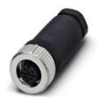
Connector, 5-position, Socket straight M12 SPEEDCON, A-coded, Screw connection, knurl material: Nickel-plated brass, cable gland Pg9, external cable diameter 6 mm ... 8 mm
