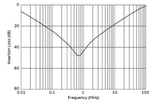
Common Mode Insertion Loss (Typ.)
