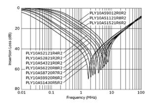
Differential Mode Insertion Loss-Frequency Characteristics
