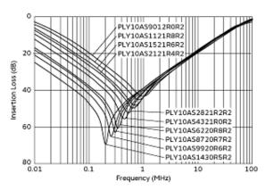
Common Mode Insertion Loss-Frequency Characteristics
