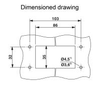
Panel cutout <sup>2)</sup> When self-tapping screws are used (Torx® 20, M4)
