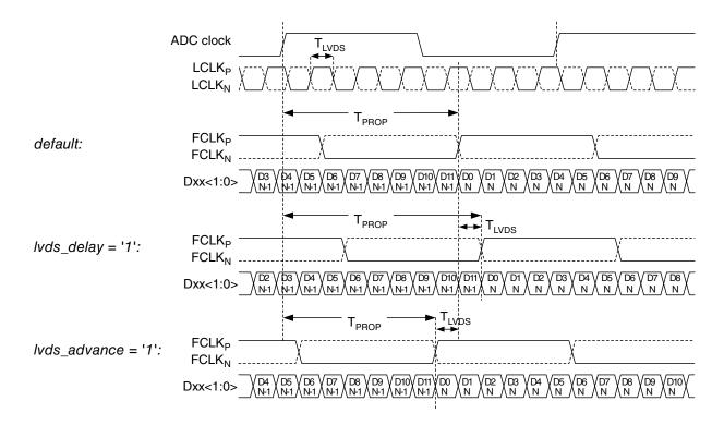
Figure 10. LVDS output timing adjustment
