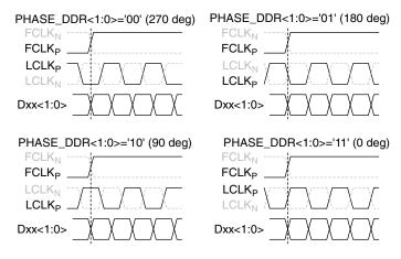
Figure 8. Phase programmability modes for LCLK
