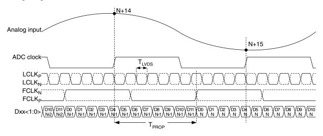
Figure 4. LVDS timing 12 bit output, DDR mode
