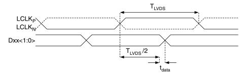
Figure 7. LVDS data timing, DDR mode
