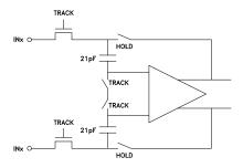
Figure 11. Input configuration
