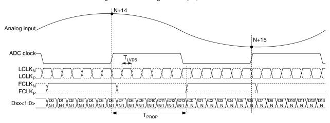
Figure 5. LVDS timing 14 bit output, DDR mode
