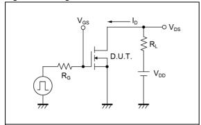
Fig.2-1 Gate Charge Measurement Circuit
