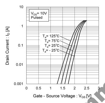
Fig.9 Gate Threshold Voltage vs.
