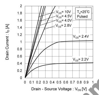
Fig.6 Typical Output Characteristics(II)
