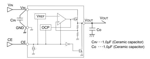
Figure 2. Block Diagrams
