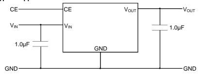
Figure 1. Application Circuit
