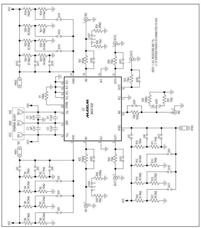
Figure 1. MAX7438 EV Kit Schematic
