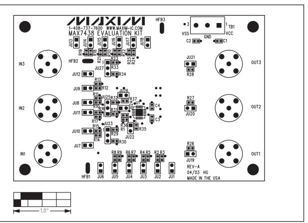
Figure 2. MAX7438 EV Kit Component Placement Guide—Top Silkscreen
