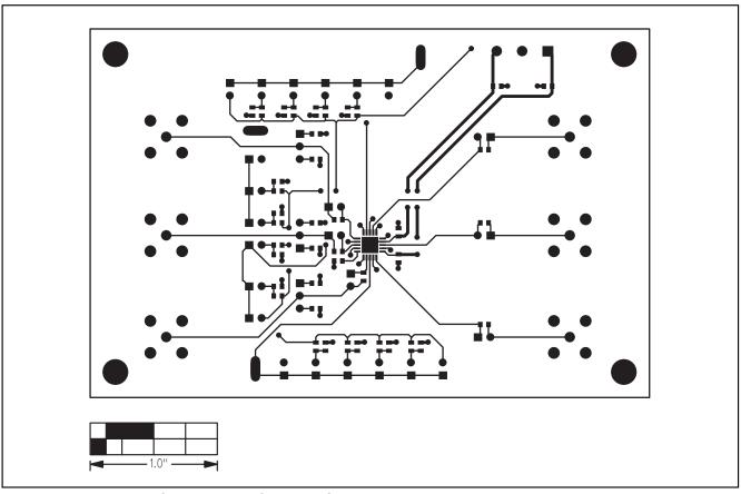
Figure 3. MAX7438 EV Kit PC Board Layout—Component Side
