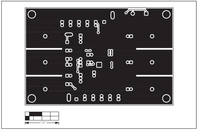
Figure 4. MAX7438 EV Kit PC Board Layout—Solder Side
