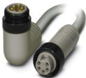
Bus system cable, DeviceNet™, 5-position, PVC, gray, Plug angled 7/8"-16UNF, A - standard, on Socket straight 7/8"-16UNF, A - standard, cable length: 15 m
