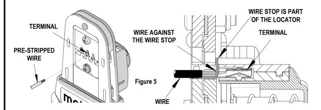
Note: The tamper proof ratchet action will not release the tool until it has been fully closed.
